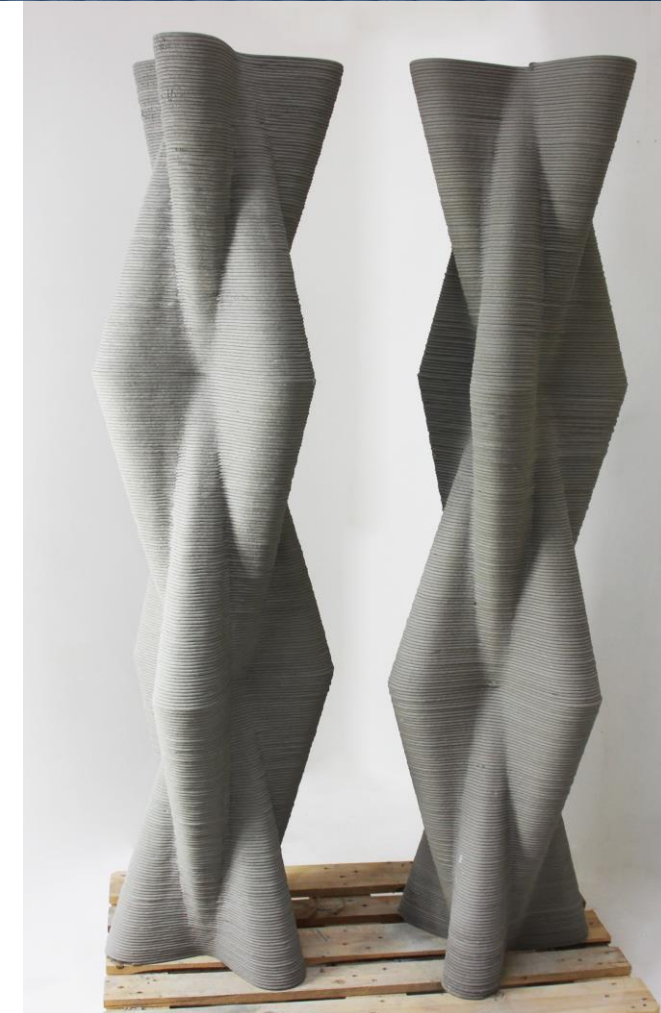
It takes 30 minutes to print a 2-meter column
